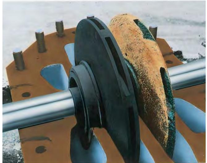
Both Impellers operated for 18 months in seawater service. However, the **SIMSITE®** Impeller is untouched by corrosion!
